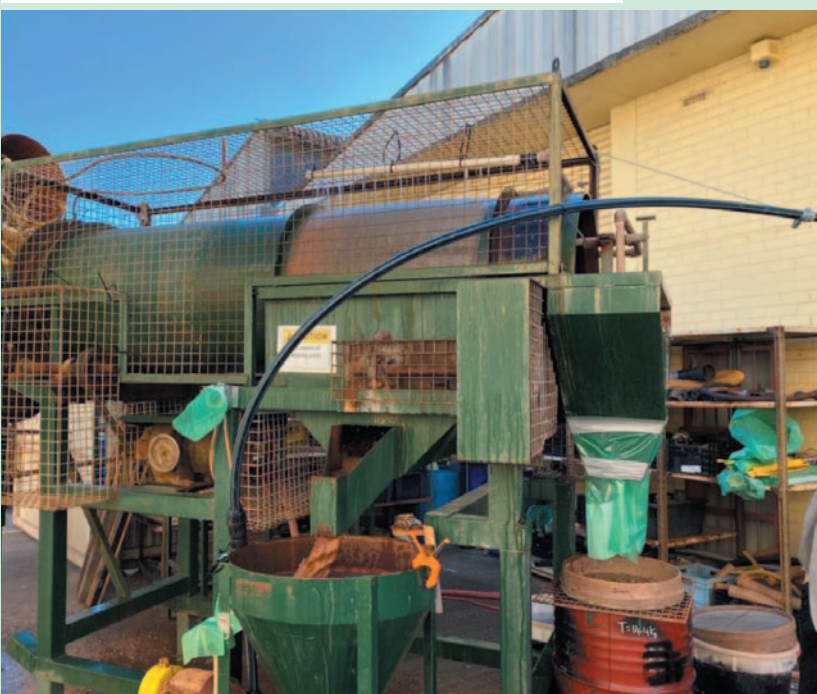
Left: Trommel screen processing the raw material & Right: +2mm oversized material
