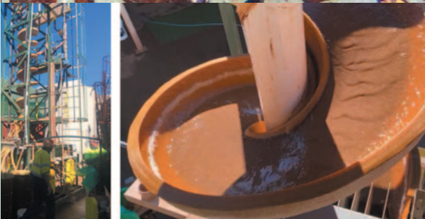
Left: Gravity spirals set-up for the processing of the deslimed and screen material & Right: Close-up of the gravity spiral in the early phases of the process
