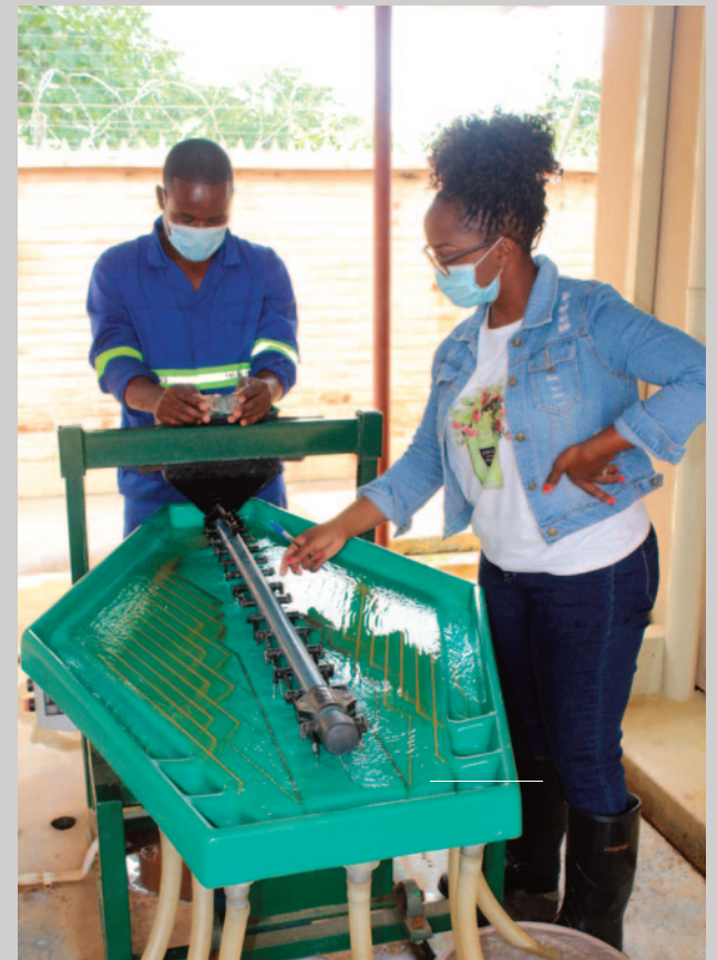
Shaking table used for separating lighter minerals from heavy minerals
