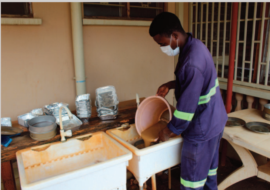
Samples are deslimed and screened in the first stage of processing
