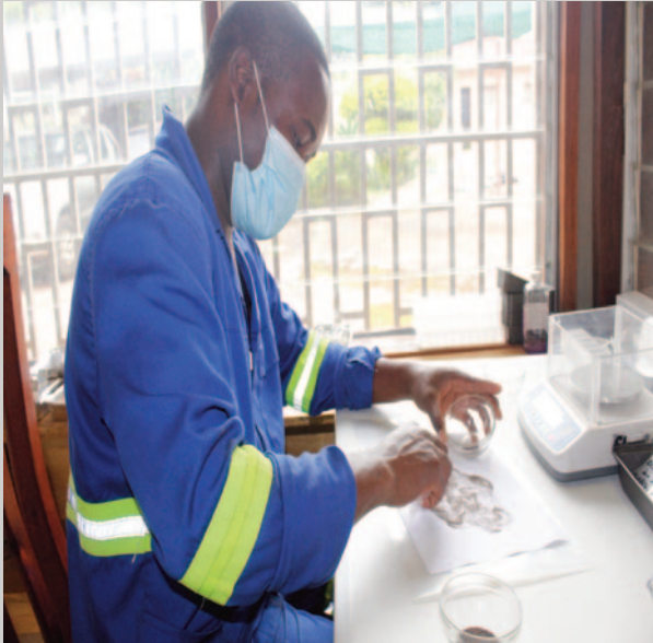
Lab Technician using a magnet to magnetically separate non-magnetic rutile from magnetic ilmenite
