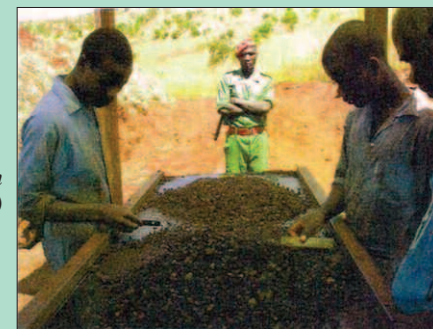
Figure 3: Sorting and grading of corundum (Source: Stuart Brand, 1977)
